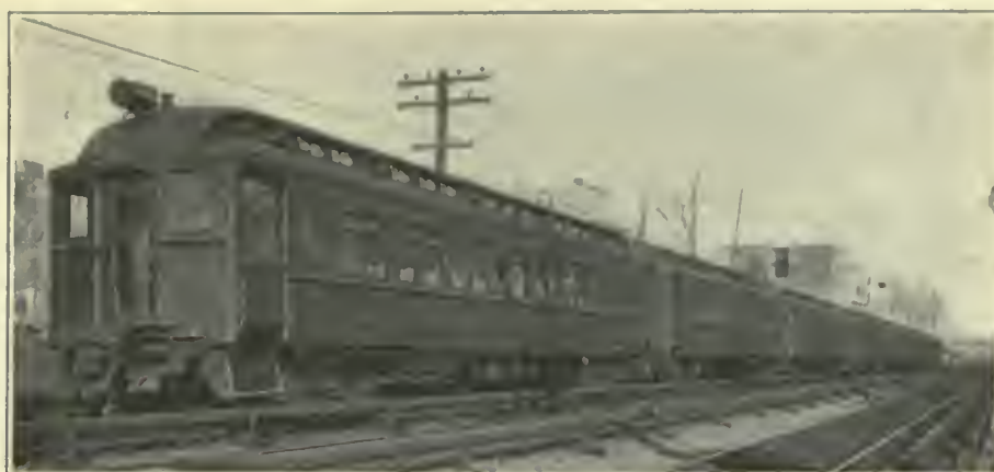
FIG. 534. MULTIPLE-UNIT TRAINS. Multiple-Unit Train for 600-Volt Direct Current Third Rail Operation, New York Central & Hudson River Railroad.
